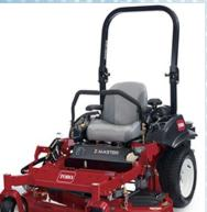
The U.S. Consumer Product Safety Commission in cooperation with The Toro Company of Bloomington, Minnesota has announced a voluntary recall of the Toro ZMaster® Riding mowers. The traction belt can wear through the mower's fuel tank and cause fuel to leak, posing a fire hazard. Approximately 2,600 units were sold nationwide at Toro dealers from January 2012 through August 2012 for between \$7,700 and \$8,700. Toro has received five reports of incidents. No injuries have been reported.
